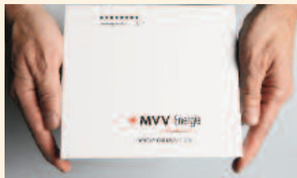
The Energiebutler® in the "Model city of Mannheim" project facilitates individual energy management, and the implementation of dynamic rates and demand-response mechanisms to switch refrigerators off, for example, if electricity is expensive or does not come from a renewable energy source.
